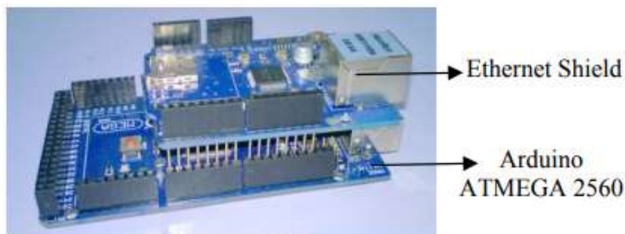
Figure 6. Ethernet shield installed on Arduino
