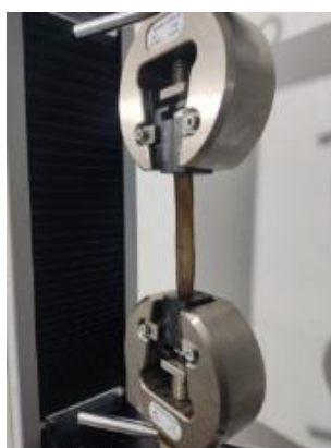
Figure 8. The process of testing the tensile strength of the sample with the instrument
