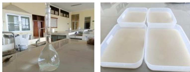
Figure 3. NaOH solution 2% (a), SB immersed in 2% NaOH solution (b)
