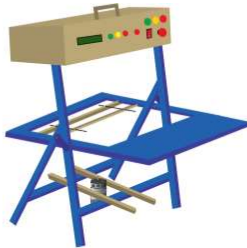
Figure 3. Design of a Microcontroller-Based Automatic Valve Cleaning Tool
