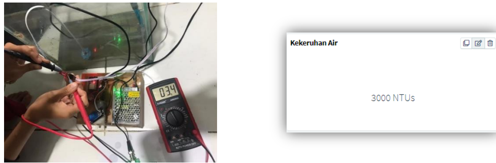
Figura.5. Voltage measurement and value display in turbid water
